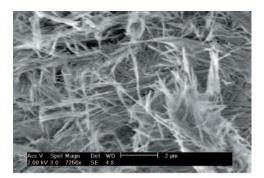
The random network of sepiolite particles holds coarser particles in the liquid preventing their settling by gravity, acting as a suspending agent. Sepiolite provides to its suspensions a pseudoplastic and thixotropic behaviour which make it a valuable material in multiple applications to improve processability, application or handling of the final product.
