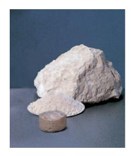
The high surface area and porosity of sepiolite account for the remarkable adsorptive and absorptive properties of this clay. It adsorbs vapours and odours and can absorb approximately its own weight of water and other liquids.
