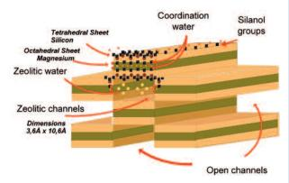
Sepiolite has the highest surface area (BET, N<sub>2</sub>) of all the clay minerals, about 300 m<sup>2</sup>/g, with a high density of silanol groups (-SiOH) which explains the marked hydrophilicity of this clay. The silicate lattice has not a significant negative charge and therefore the cation exchange capacity of this clay is very low.
