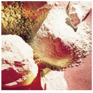
a fine-grained igneous rock with the same mineralogical composition as granite is also frequently mined for its feldspar content.
